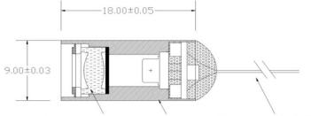
Aspherical plastic lens Copper case Power Lead (~ 150mm)
